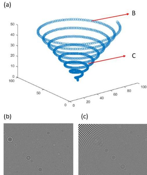
FIGURE 3. Illustration of an arbitrarily generated scanning path for TPP; the holograms of two different points on the scan path (B and C) are shown in Fig. 3B and 3C, respectively.
