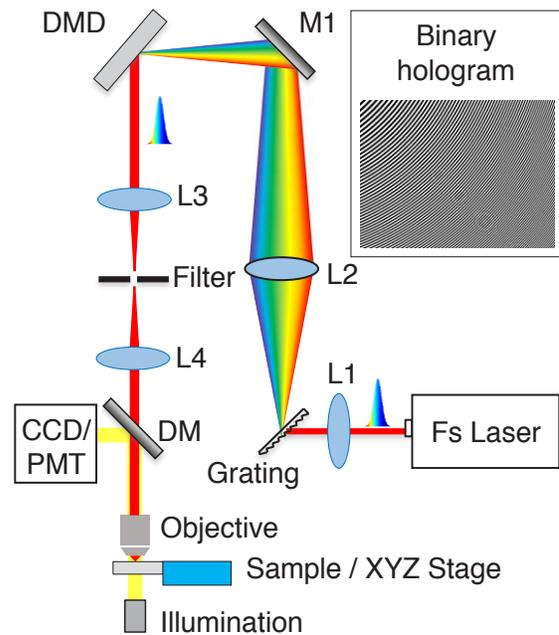
FIGURE 1. Optical configuration of the TPP fabrication system and TPE imaging system, enabled by DMD random-access scanner; M1, M2: high-reflectivity mirrors; DM: dichroic mirror; L1, L2, L3, and L4: lenses
