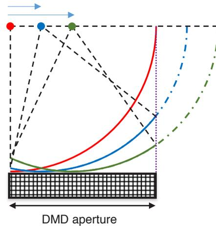
FIGURE 2. Working principle of lateral scanning based on binary holography: The focal point can be scanned from left (red) to right (green) by reducing the value of the tilted phase term, i.e.,  $R(x,y)/T$ , in Eq. (2), i.e., reducing the value of  $R(x,y)$  when  $T$  (grating period) is constant.
