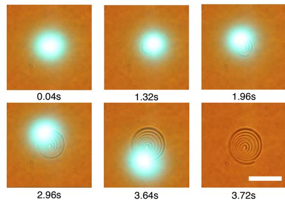
FIGURE 4. Time sequence of the spiral scanning and fabrication process performed by the DMD holography scanner. Scale bar is  $25 \mu\text{m}$ .
