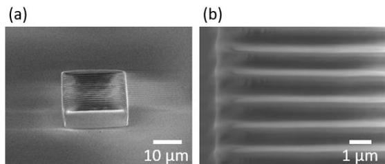
**FIGURE 5.** DMD illustration of fabricated structures via TPP: (a) SEM image of printed straight lines with 0.4/1.2  $\mu$ m linewidth/pitch on a  $20 \mu\text{m} \times 20 \mu\text{m}$  cube substrate. (b) Zoomed SEM image of printed straight lines.
