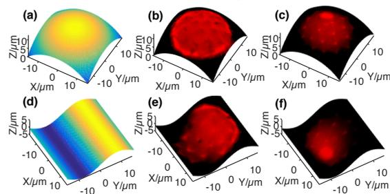
**FIGURE 6.** Cross-sectional images of two selected pollen grains on arbitrarily programmed spherical and sinusoidal surfaces
