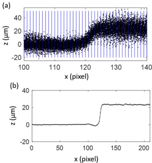
FIGURE 5. Resampling the slanted stepped surface: (a) superimposed step profiles where each profile is aligned along the step edge; the vertical lines show the sampling intervals. (b) The averaged step profile.
