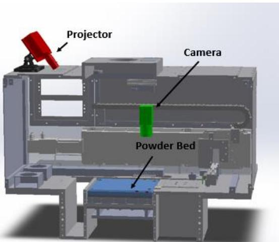
FIGURE 2. An in-situ fringe projection system for a LPBF machine (some parts are hidden for clear visualization).
