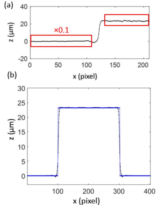
FIGURE 6. Further noise reduction on the averaged step profile: (a) The noise on the lower and upper surfaces are reduced by multiplying by a small coefficient. (b) The measured step profile (black) and the mathematically perfect step profile (blue) are duplicated and folded to form double-sided step profiles.
