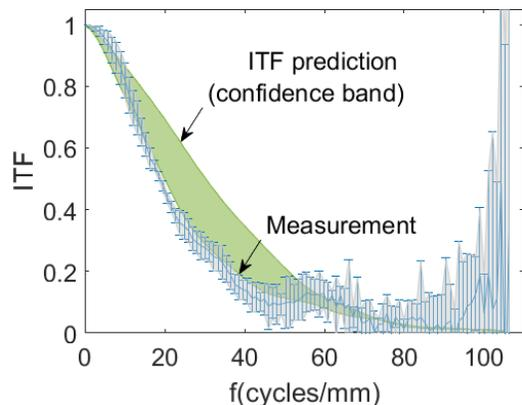
FIGURE 7. The measured ITF compared with a theoretical ITF prediction.
