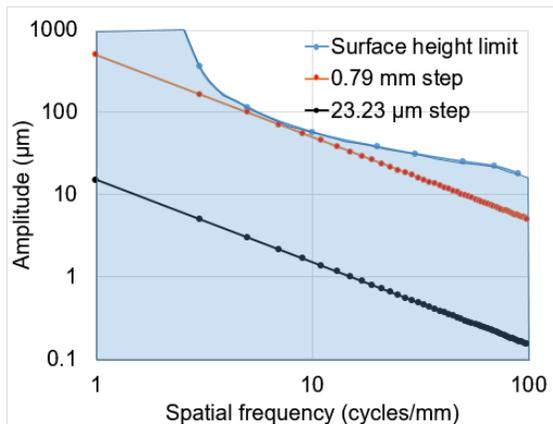
FIGURE 3. The surface height limit defines the maximum amplitude for each spatial frequency component of a measured surface for the system to behave approximately linear. A 23- $\mu\text{m}$  stepped surface is below the linearity limit.
