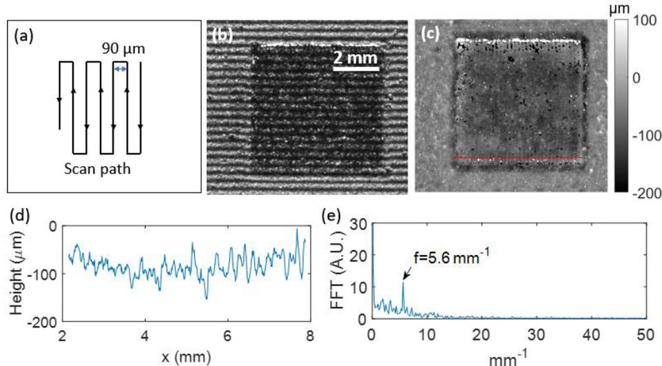
FIGURE 1. A fused square on a layer of Inconel-625 metal powder created by the LPBF process: (a) laser scan path, (b) sinusoidal fringe pattern on a fused layer of powder, (c) the height map of the fused powder layer, (d) a cross-section profile near the bottom edge of the fused region, and (e) the Fourier spectrum of the line trace.
