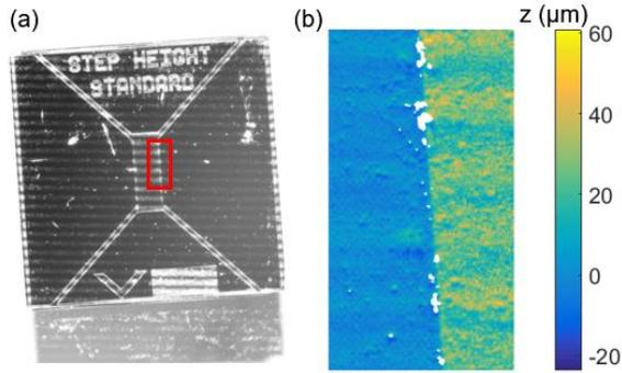
FIGURE 4. Measuring a 23- $\mu\text{m}$  stepped surface with fringe projection: (a) the fringe pattern on the stepped surface, and (b) the measured height map of the outlined region.
