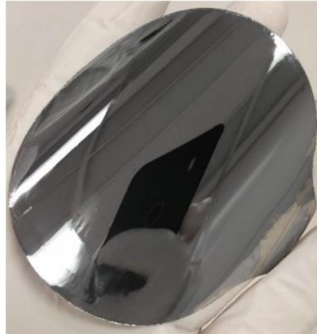
FIGURE 3. Exfoliated film sample. Silicon side up with nickel backing.
