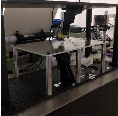
FIGURE 4. KEYENCE differential laser displacement thickness measurement system.
