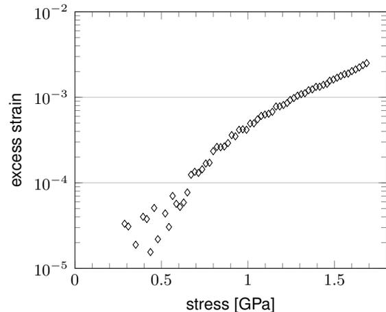
FIGURE 2. Excess strain of an Elgiloy® wire as a function of applied stress. Values below  $5 \times 10^{-5}$  reflect measurement noise.
