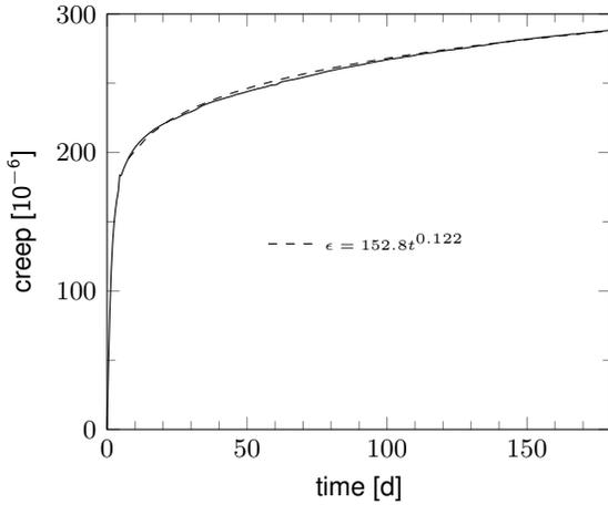
FIGURE 3. Initial creep of an Elgiloy® wire under 993 MPa axial stress with best-fit Bailey-Norton creep curve.
