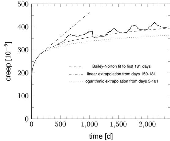
FIGURE 5. Long-term creep of an Elgiloy® wire under 993 MPa axial stress with Bailey-Norton, linear, and logarithmic creep extrapolations based on the first 181 days of data.
