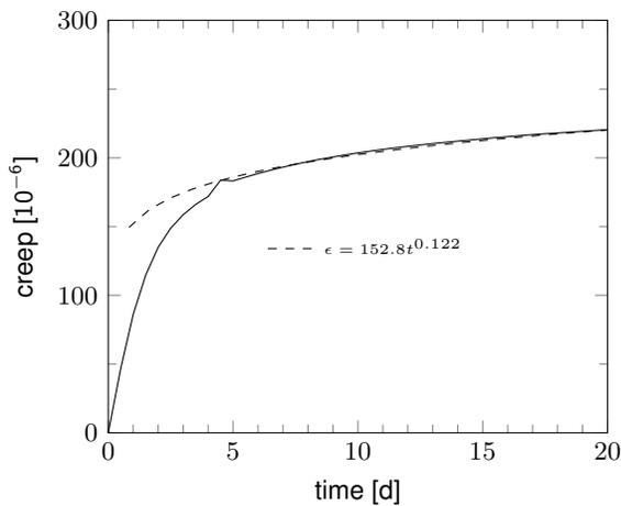
FIGURE 4. Early creep of an Elgiloy® wire under 993 MPa axial stress with best-fit Bailey-Norton creep curve, showing anelastic settling during the first five days.
