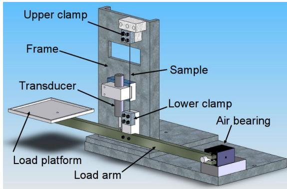
FIGURE 1. Apparatus used to measure long-term creep of wires under axial load.
