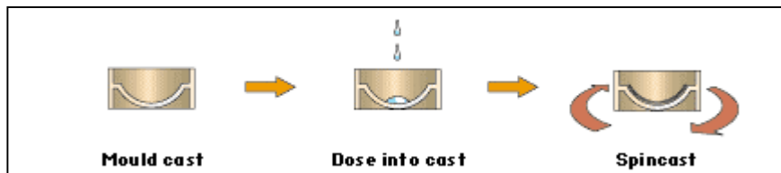
Principle of Spin Casting Contact Lens
